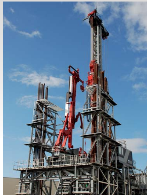
Pipe handling system and vertical storage
