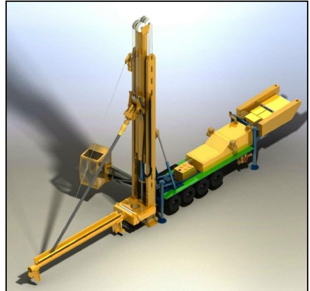
Semi-trailer with pipe handling system
